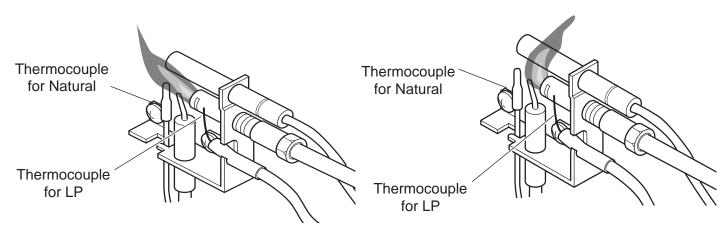
Figure 30 - Correct Appearance of Pilot Flame
